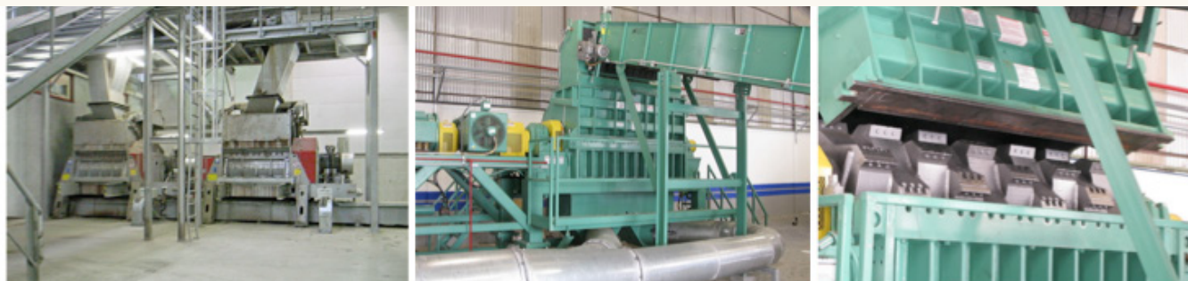
Figure 20: Secondary Shredding Mill in Austria (left) and Mexico (center and right)
